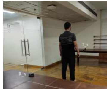
Fig. 1: System setup for detection of standing human, distance between Transceiver ( T_x ) and Receiver ( R_x ) is 4m
